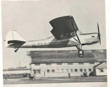
The Auster Avis four-place personal aircraft powered by a de Havilland Gipsy Major 10 four-cylinder engine of 145 b.h.p.
